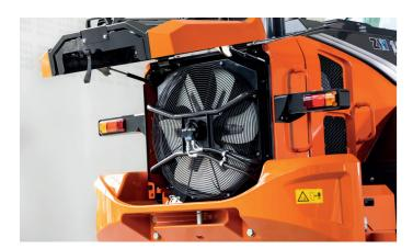
Intelligent fan operation system prevents radiators clogging.
