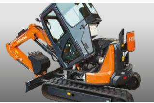
The tilting floor enables easy access to the engine and control valve for quick servicing.
