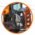
**Easy maintenance** The radiator and oil cooler are conveniently positioned side by side.
