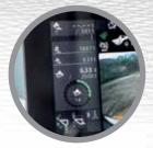
The payload checker helps you work more productively and accurately when loading trucks.
