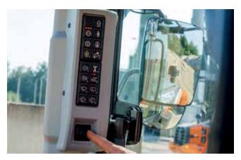
Electrically adjusted mirrors provide a clear rear view.
