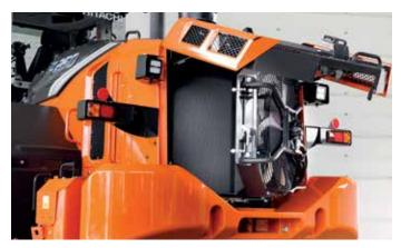
Intelligent fan operation system prevents radiators clogging.
