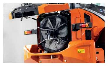
Intelligent fan operation system prevents radiators clogging.
