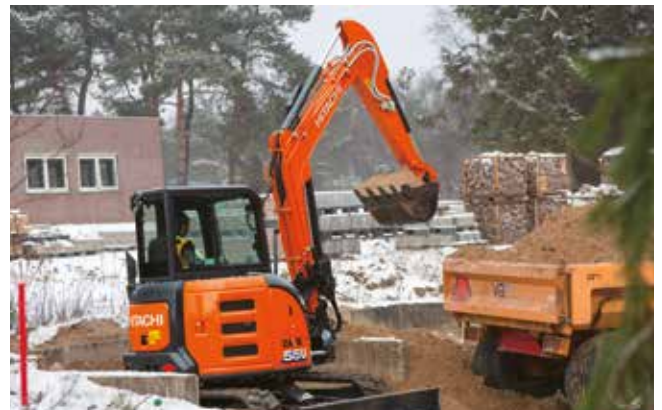
The short-tail swing radius makes the ZX55U-6 ideal for working in tight spaces.
