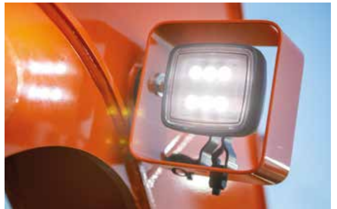
LED lights have a longer lifetime than halogen alternatives.
