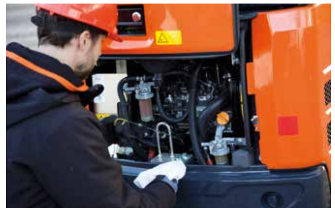
Daily inspection points are grouped together for convenience.
